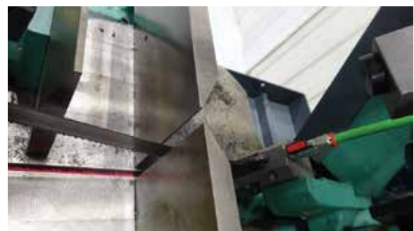
Laser pointer for cutting position
