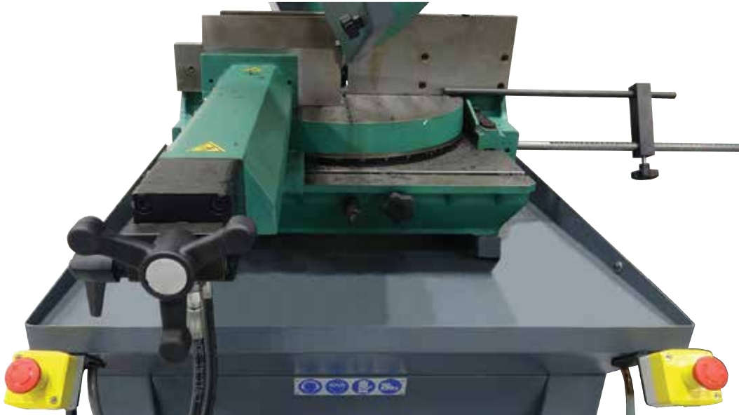
Vise with quick approach, can be positioned transversally along the entire machine base. Adjustable vise shoulders.
