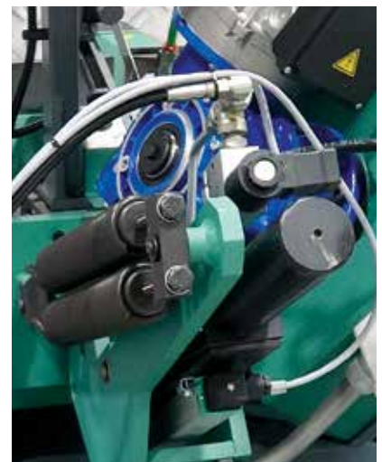
Hydraulic cylinder for bow movement
