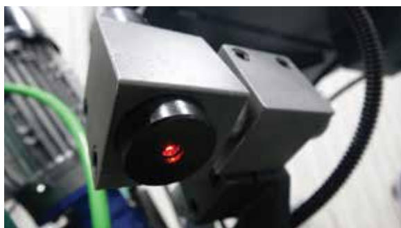
Laser pointer for cutting position
