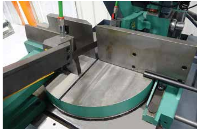
Large circular table rotating together with the bow to ensure optimal support of the piece to be cut.
