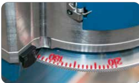
Degree wheel for repeatable bending angles
