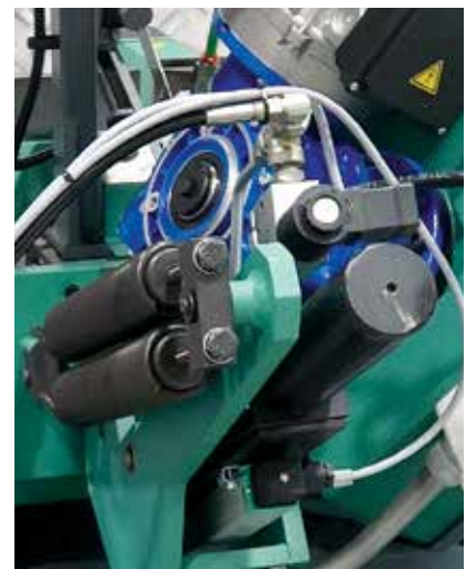
Hydraulic cylinder for bow movement
