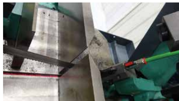
Laser pointer for cutting position
