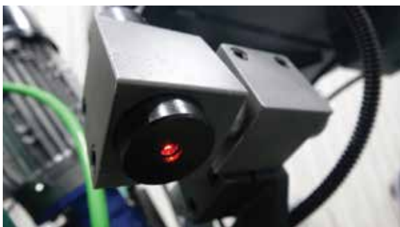
Laser pointer for cutting position
