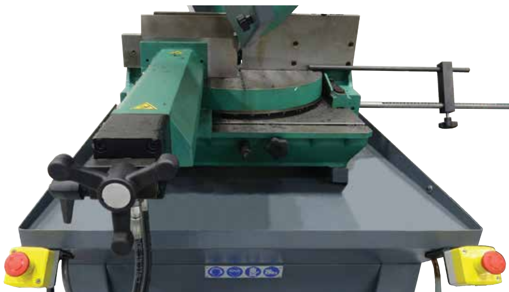
Vise with quick approach, can be positioned transversally along the entire machine base. Adjustable vise shoulders.
