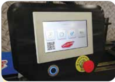
Easy touch screen bend angle programming.
