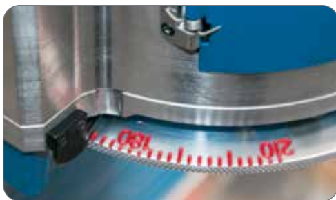
Degree wheel for repeatable bending angles
