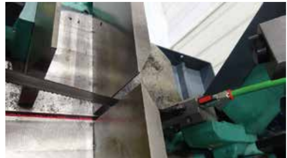
Laser pointer for cutting position
