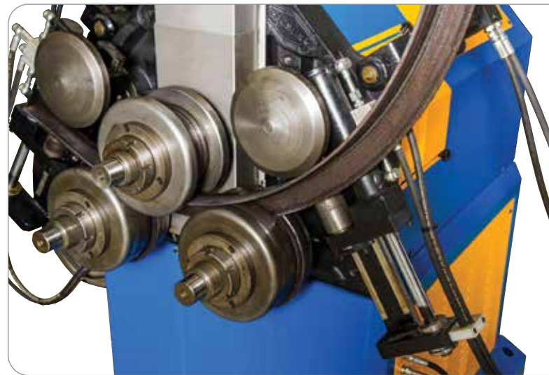
CE70H3-RLI w/Hydraulic 3 Axis Twist
