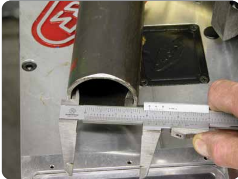
Pipe dimensions are based on I.D. of material (2" sch. 40 pipe measures 2.375" O.D.).
