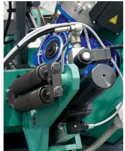
Hydraulic cylinder for bow movement
