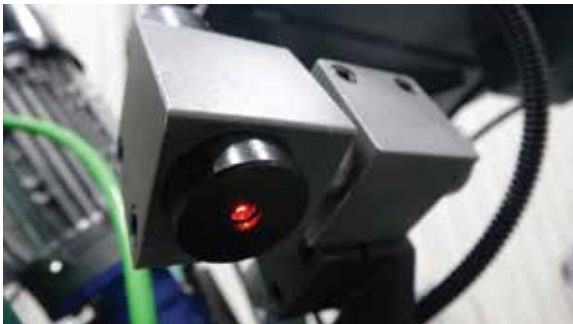
Laser pointer for cutting position
